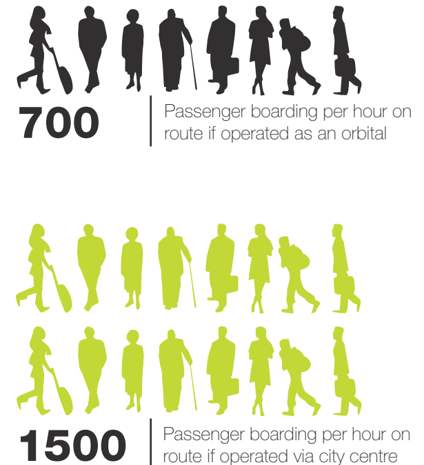
Figure 3.5 Modelled Boardings Comparison for Radial and Orbital cross-city services (AM Peak boardings in both directions)
