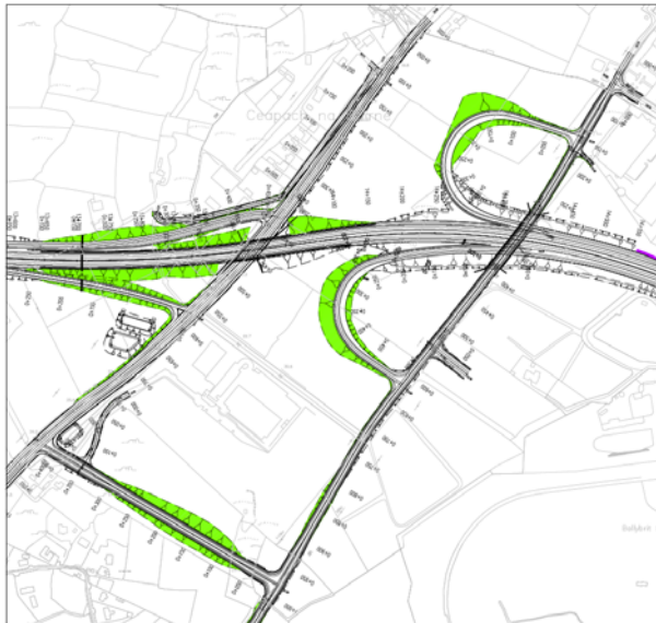
Figure 23: Refined N17 and Parkmore Link Road Junction November 2016
